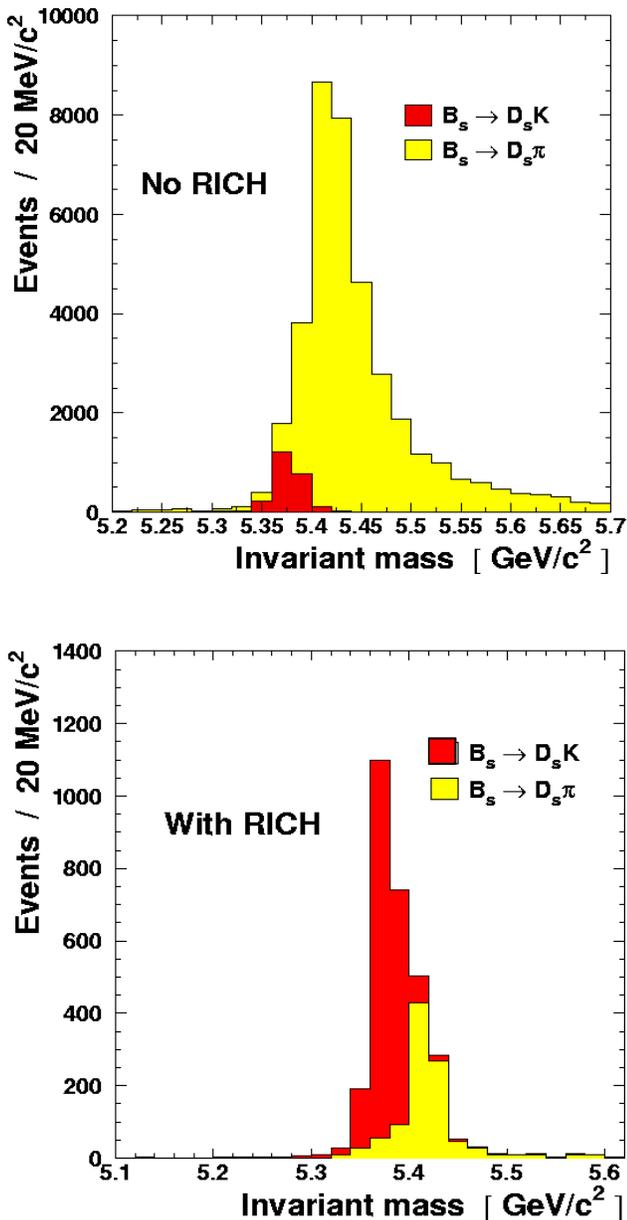
**Figure 3.** Without particle identification from the Cherenkov detectors in a simulation from LHCb (top) the  $B_s \rightarrow D_s^- K^+$  signal is drowned by the  $B_s \rightarrow D_s^- \pi^+$  decay. With particle identification (bottom), the signal is dominant compared to the background.
