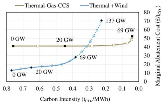
Fig. 4. Carbon abatement cost as a function of the resulting power system carbon intensity for a thermal-wind and thermal-gas-CCS integrated power system.
