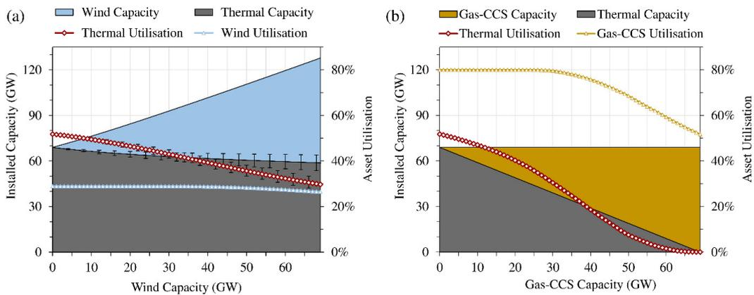
Fig. 2. Capacity share and power plant utilization factor for (a) a thermal-wind integrated system, and (b) a thermal-gas-CCS integrated system as a function of the amount of wind and gas-CCS capacity deployed, respectively. Underlying data on wind availability in the UK is from Staffell and Green [39]. The error bars shown in (a) refer to high (+ 5-10%) and low (- 5-10%) estimates of the wind capacity credit.
