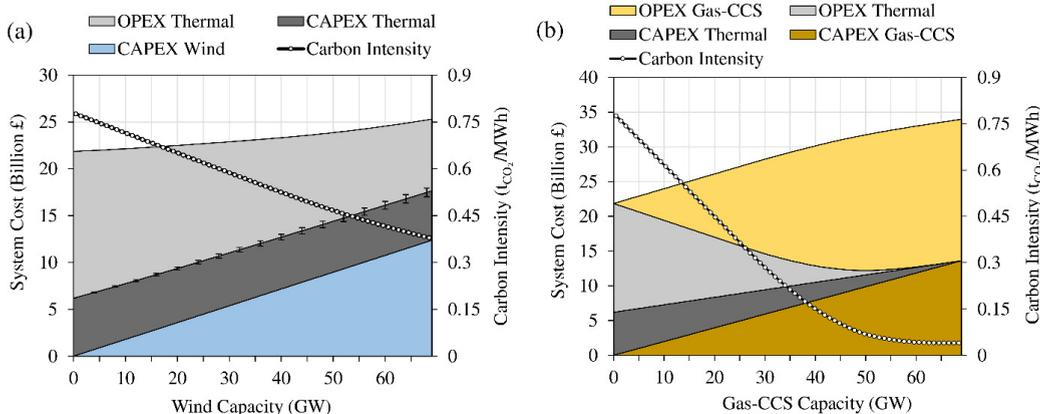
Fig. 3. Total system cost and Carbon Intensity for (a) thermal-wind integrated system, and (b) a thermal-gas-CCS integrated system depending on the wind and gas-CCS capacity deployment level, respectively. Data source and error bar indication are analogous to figure 2.
