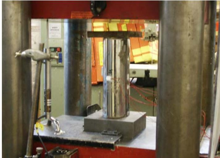
Figure 3: Test set-up for EHS composite column
