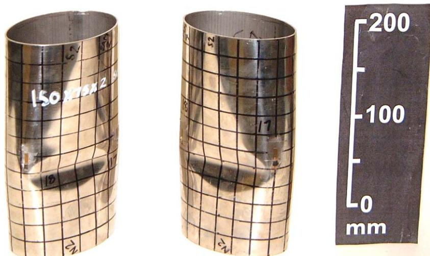
Figure 4: Mode of failure of the unfilled EHS columns
