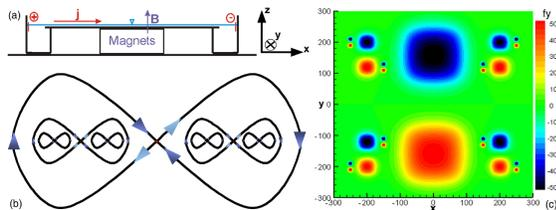
FIG. 1: (a) Schematic of rig; (b) Schematic of multi-scale flow based on a 8 in 8 topology, (c) Electromagnetic forcing distribution computed for our spatial distribution of multi-sized magnets ( $I=1A$ ,  $B=1T$ ;  $f_y$  in  $N/m^3$ ;  $x$  and  $y$  in  $mm$ ).
