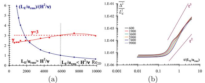
FIG. 5: (a) Richardson-like exponent,  $\gamma$ , ( $\overline{\Delta^2} \sim t^\gamma$ ) and ratio  $L_E/u_{rms}$  to  $H^2/\nu$  as function of  $Re_{2D}$ ; (b) two-particle dispersion,  $\overline{\Delta^2}/L_E^2$ , various  $Re_{2D}$ .
