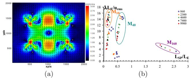
FIG. 2: (a) PIV velocity field ( $\mathbf{u}/u_{rms}$ ,  $1/64$  arrows),  $Re_{2D} = 600$ , squares refer to hyperbolic stagnation points, disks to elliptic stagnation points; (b) scatter plot of hyperbolic stagnation point strain rates,  $\lambda L_E / u_{rms}$ , and sizes,  $L_S / L_E$ .
