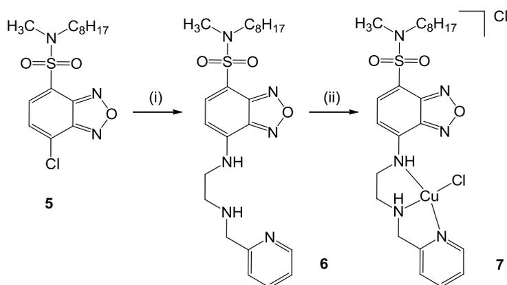
**Scheme 2.** Synthetic scheme for the preparation of ligand **6** and the corresponding Cu complex **7**. (i) Under N<sub>2</sub>, dry acetonitrile, NEt<sub>3</sub>, H<sub>2</sub>NCH<sub>2</sub>CH<sub>2</sub>NHCH<sub>2</sub>Py; (ii) Methanol/Acetonitrile, CuCl<sub>2</sub>.
