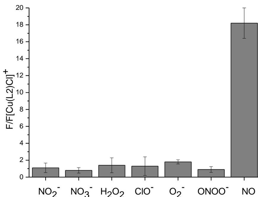
**Figure 2.** Emission intensity (recorded at 580 nm) of 10  $\mu\text{M}$  solutions of complex **7** after addition of 100 eq. of  $\text{NO}_2^-$ ,  $\text{NO}_3^-$ ,  $\text{H}_2\text{O}_2$ ,  $\text{ClO}^-$ ,  $\text{O}_2^-$  and  $\text{NO}$  and incubating for 1 hour in buffered PBS (pH 7). Average emissions (triplicate  $\pm$  SD) were normalised with respect to the emission of **7** (10  $\mu\text{M}$ ).
