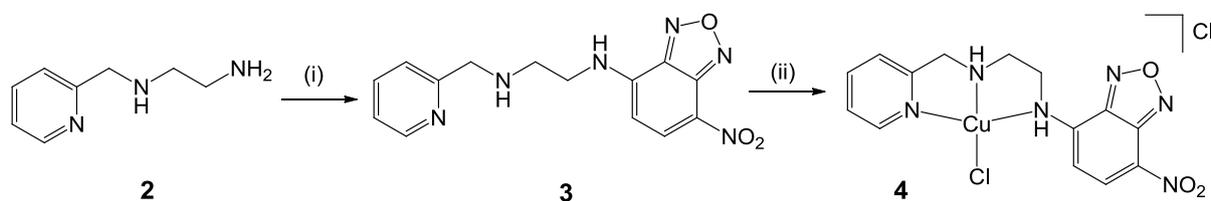
**Scheme 1.** Synthetic scheme for the preparation of ligand **3** and the corresponding copper(II) complex **4**. (i) Dry methanol,  $K_2CO_3$ , NBD-Cl; (ii) Methanol,  $CuCl_2$ .
