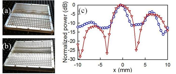
Fig. 5. Fabricated prototypes with  $q=0$  (a) and  $q=0.35$  (b). (c) Experimental results of the normalized power distribution along the transversal  $x$ -axis at each  $FL$  for the zoned fishnet metalenses with  $q = 0$  (circles) and  $q = 0.35$  (triangles).
