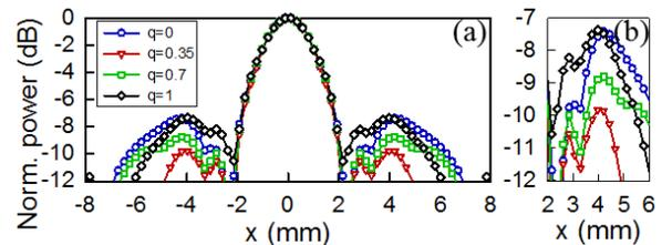
Fig. 4. (a) Numerical results of the normalized power distribution along the transversal  $x$ -axis at each numerical  $FL$  for the zoned fishnet metalenses with  $q = 0$  (circle),  $q = 0.35$  (triangles),  $q = 0.7$  (squares) and  $q = 1$  (diamonds). (b) Zoom-in of the SLL from (a).
