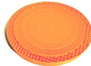
Fig. 2. Ku-band FDM graded index flat lens [4].
