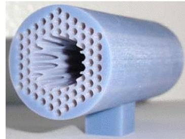
Fig. 7. 146 GHz polyjet EXMT waveguide horn [8].
