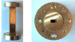
Fig. 9. E-Band SLM band pass filter [9].
