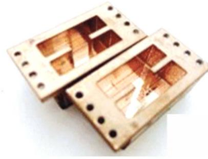
Figure 5: X-Band polyjet band-pass filter [7].
