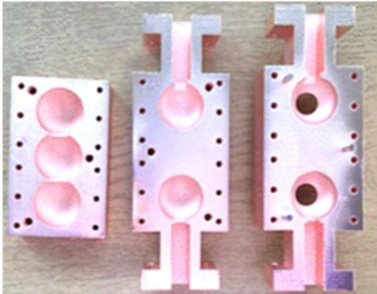
Fig. 4. X-Band FBM split block spherical cavity filter [6].
