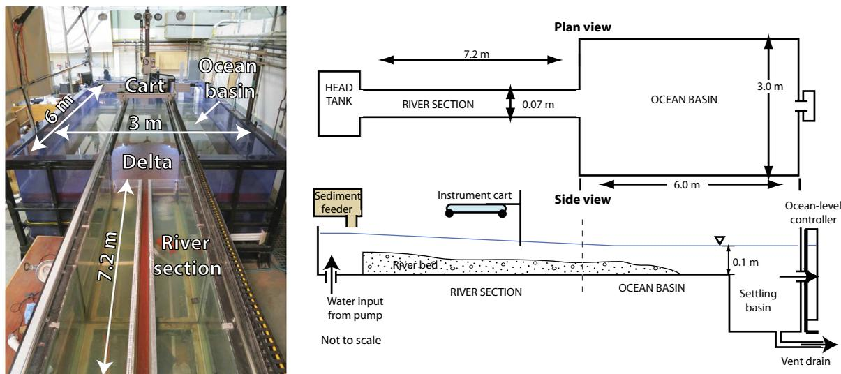
**Fig. 2. Experimental arrangement at Caltech Earth Surface Dynamics Laboratory.** Schematic of the experimental arrangement along with a perspective photograph showing the alluvial river section, ocean basin, and the instrument cart, which was used to collect water surface and bed elevation data during both experiments.
