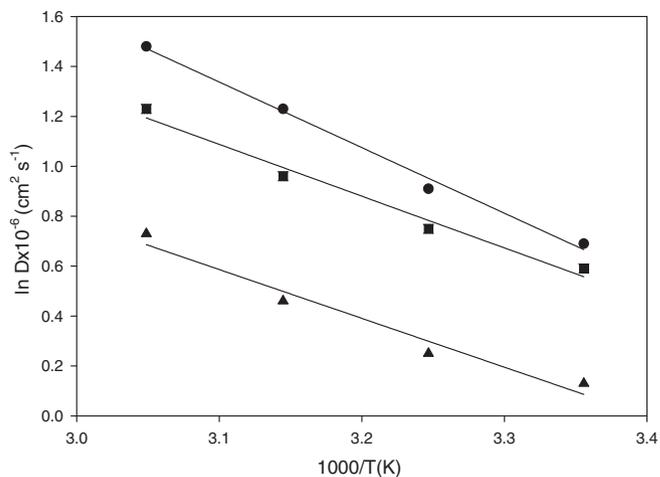
**Figure 6.** The plot of  $\ln D$  versus  $1/T$  based on the cathodic peak currents for the V(III)/V(IV) redox couple on the GC electrode in DES3, DES8 and DES10.
