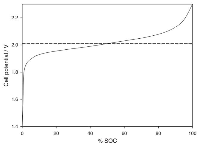
**Figure 5.** Plot of the Nernst equation for a single-electron disproportionation reaction with a 2.01 V cell potential (DES3).
