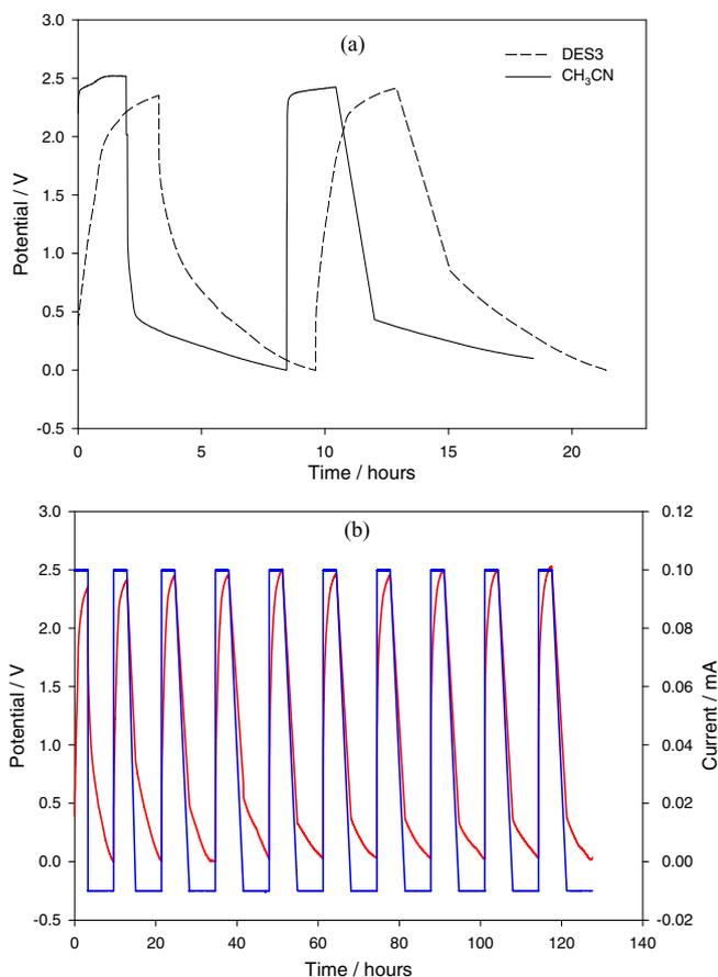
**Figure 7.** (a) Charge/discharge curves for (0.01 M  $V(acac)_3/0.5$  M TEABF<sub>4</sub> in  $CH_3CN$  (the charge current was 1 mA and the discharge current was 0.1 mA) AND charge/discharge curves for 0.01 M  $V(acac)_3/0.5$  M TEABF<sub>4</sub> in DES3 (the charge current was 0.1 mA and the discharge current was 0.01 mA); (b) Charge/discharge curves during the 3<sup>rd</sup> and 12<sup>th</sup> cycles for 0.01 M  $V(acac)_3/0.5$  M TEABF<sub>4</sub> in DES3.
