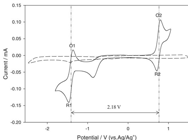
**Figure A1.** Cyclic voltammograms recorded at a glassy carbon electrode in 0.5 M TEABF<sub>4</sub> in CH<sub>3</sub>CN (---) and 0.01 M V(acac)<sub>3</sub> with 0.5 M TEABF<sub>4</sub> in CH<sub>3</sub>CN (—) at 0.1 V s<sup>-1</sup>. This result is similar to that reported in the literature.<sup>31</sup>
