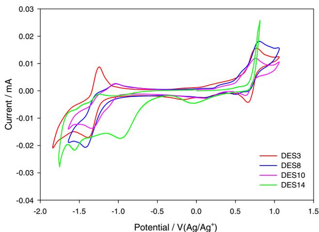
**Figure 3.** Cyclic voltammograms recorded at  $0.1 \text{ V s}^{-1}$  at a glassy carbon electrode in  $0.01 \text{ M V(acac)}_3$  and  $0.5 \text{ M TEABF}_4$  in DES3, DES8, DES10 and DES14.
