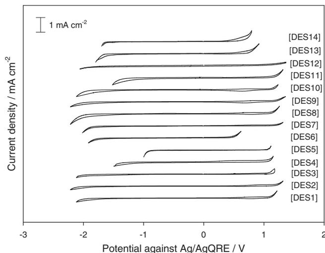
**Figure 2.** PWs of DESs based on ammonium and phosphonium salts and different HBDs. Experiments were performed using cyclic voltammetry with a glassy carbon working electrode at a scan rate of  $0.1 \text{ V s}^{-1}$ . Similar results are reported in our earlier publications and reproduced with permission from RSC, Elsevier and ECS respectively.<sup>27,30</sup>
