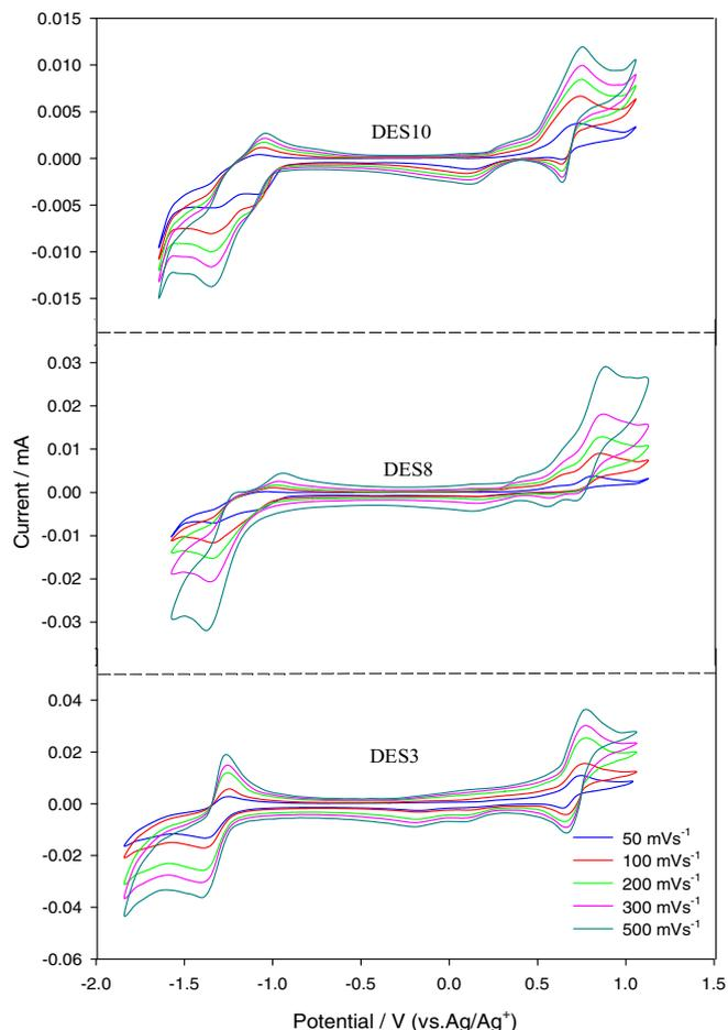
**Figure 4.** Cyclic voltammograms for  $0.01 \text{ M V(acac)}_3/0.5 \text{ M TEABF}_4$  in DES3, DES10 and DES8 using a glassy carbon electrode at a range of scan rates.
