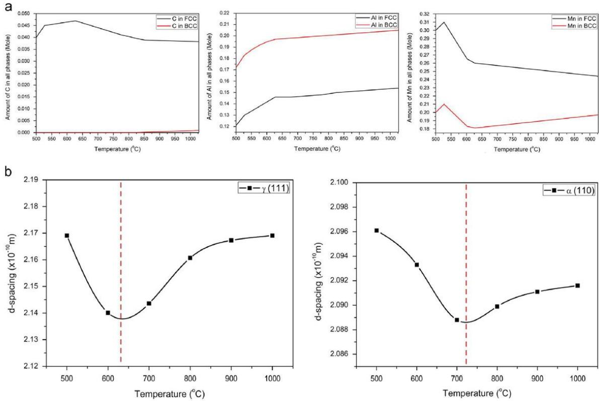
**FIG. 4** (a) Calculated equilibrium concentration of C, Mn, and Al in ferrite and austenite by Thermo-Calc software. (b) The progression of the measured austenite (111) and ferrite (110)  $d$ -spacing values as a function of temperature.
