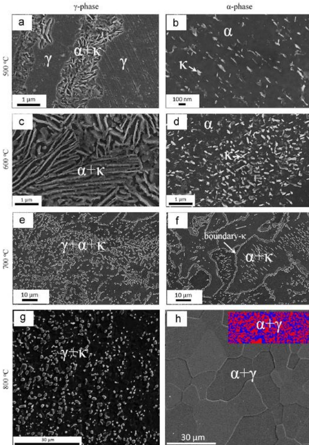
**FIG. 1** SEM and EBSD micrographs illustrating the microstructural evolution in steels within the temperature range 500–800 °C.
