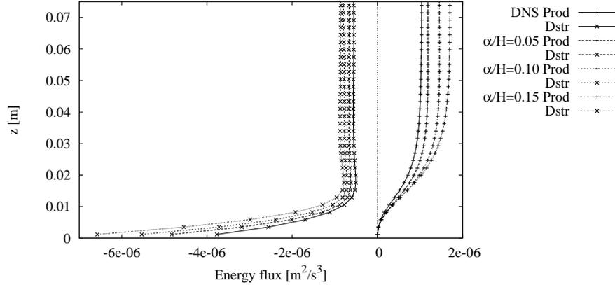
**Fig. 2.** production  $\mathcal{P}$  (Prod) and dissipation  $\varepsilon$  (Dstr) of turbulent kinetic energy as a function of  $z$ .
