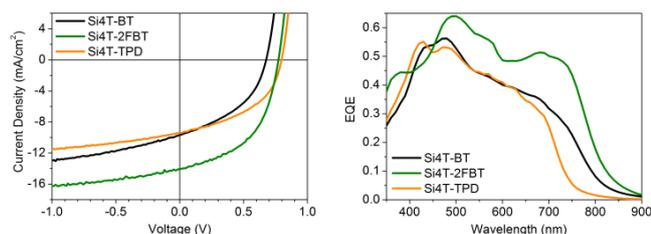
**Figure 2.** J-V curve (left) and external quantum efficiencies spectra (right) of **Si4T**-polymer:PC<sub>71</sub>BM OPV devices.
