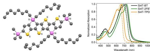
Figure 1. Single crystal structure of compound **5** (left). Normalized optical absorption spectra of Si4T polymers (right) in dilute chlorobenzene (CB) solution (dashed lines) and as thin films (full lines) spin-cast from CB solution.
