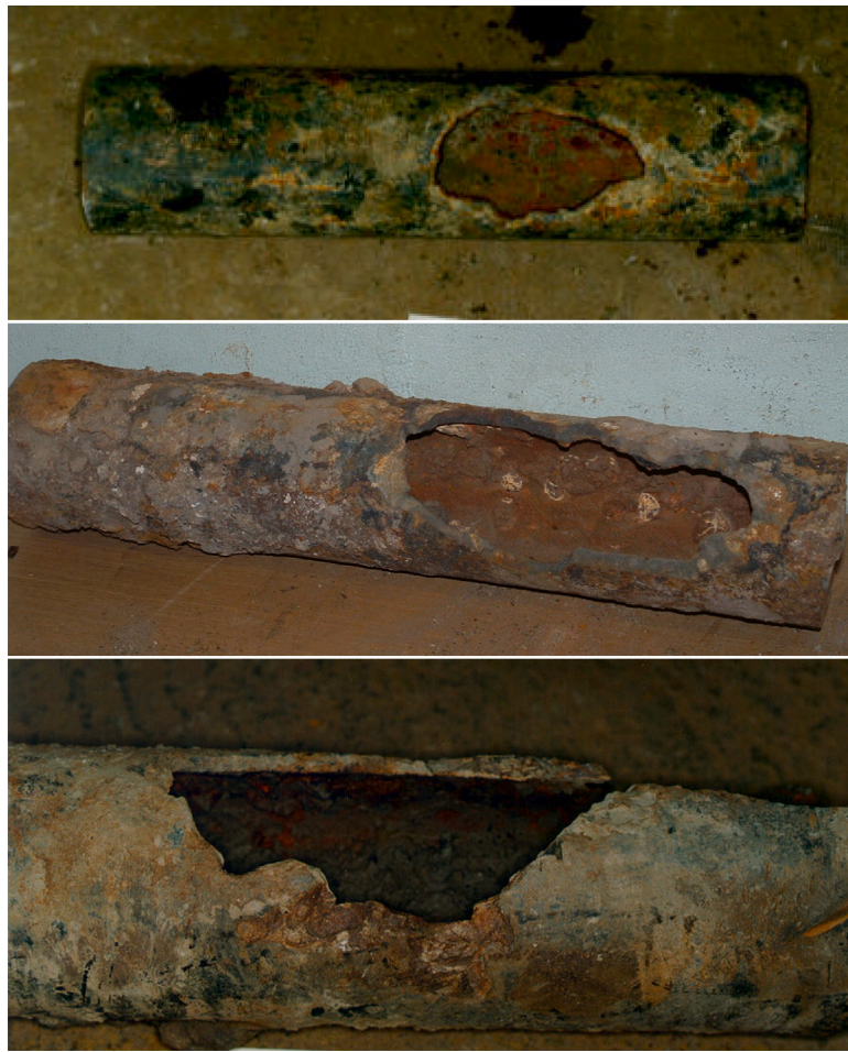
Fig. 9. Examples of cast iron pipe blowouts. Samples provided by Bristol Water, UK.
