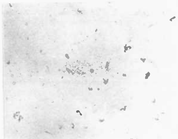
Figure 2.8 Electron micrograph of soot particles collected from flame.
