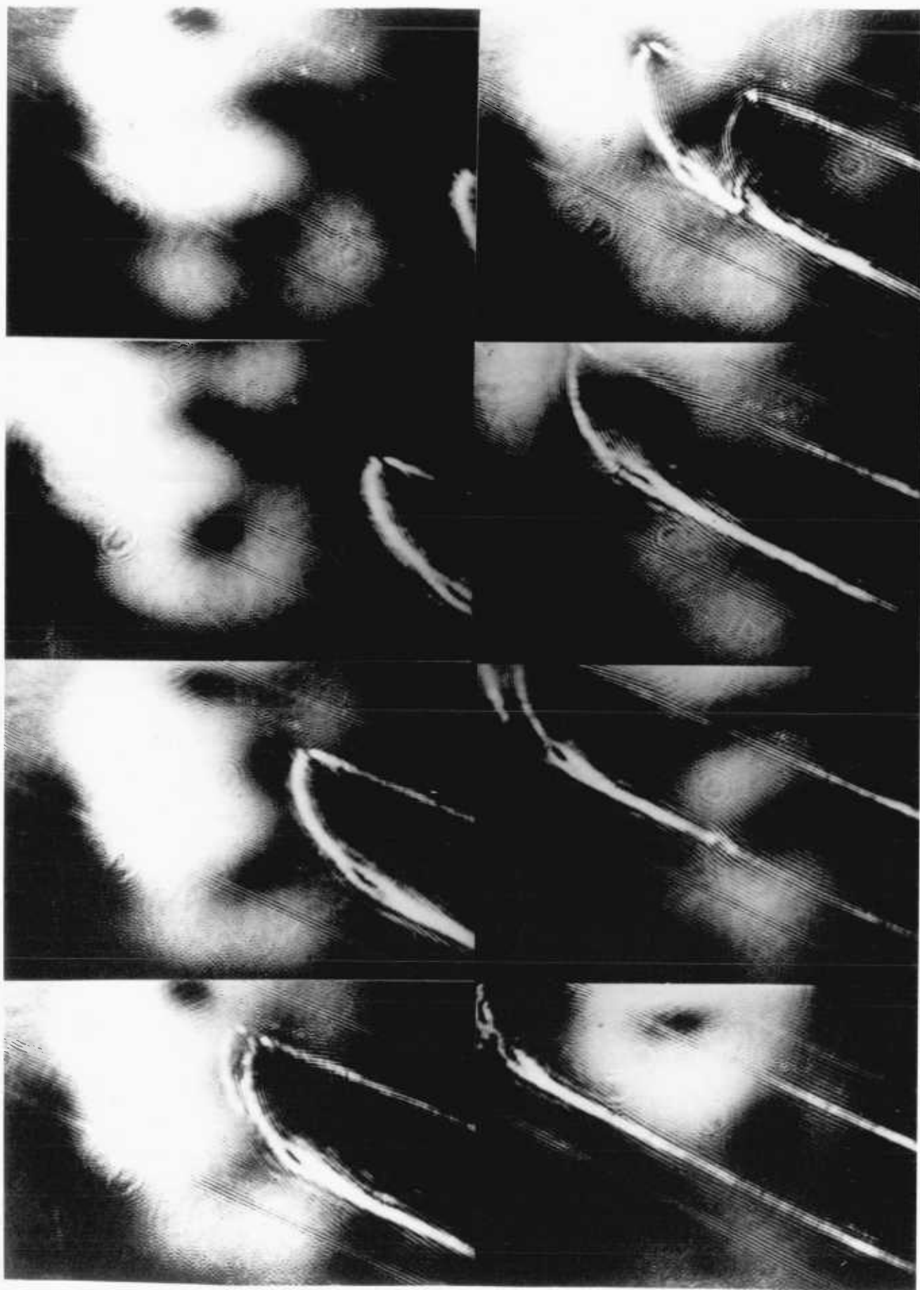
Figure 4.17 A high speed cine sequence of fringe pattern for a flame propagating down a tube
