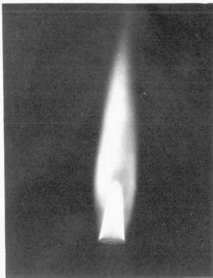
Figure 4.22a A burner-stabilized premixed flame
