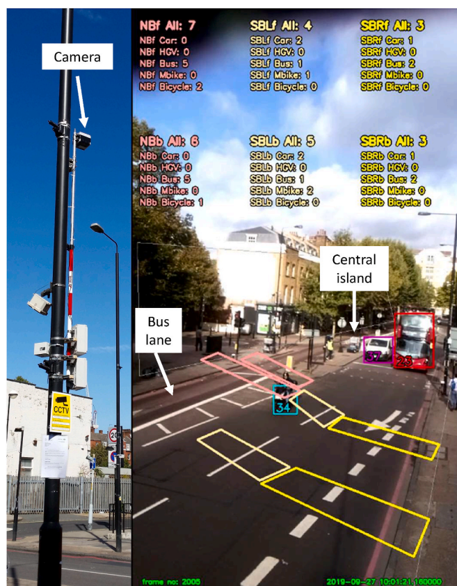
Fig. D.6. Image of one of the cameras attached to a lamppost and frame from video footage showing traffic counting areas on each lane and cumulative traffic counts. Mbike stands for motorbike, NBf stands for front counter on the NB lane and NBb for the back counter. Similarly for the other lanes. SB stands for southbound.
