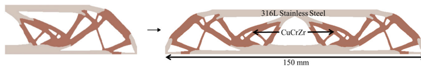
Fig. 4. Resultant multi-material (316 L stainless steel & CuCrZr) MBB beam designed through the AAP algorithm, with the objective of minimizing mechanical compliance.
