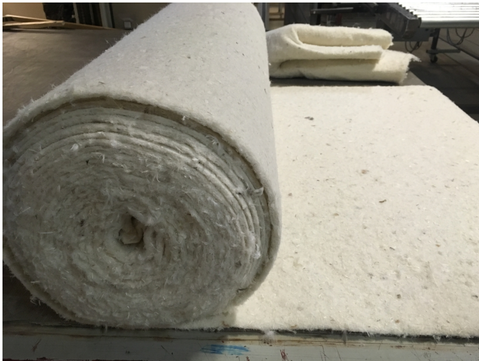
Fig. 4. Typical air laid non-woven feather fibre composite material.
