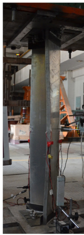
(b) Flexural-torsional buckling mode
