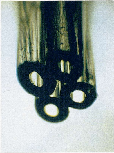
Figure 2.2 The four bore tip from which the stock solutions are dispensed. The diameter of the four bore tube is approximately 1mm.
