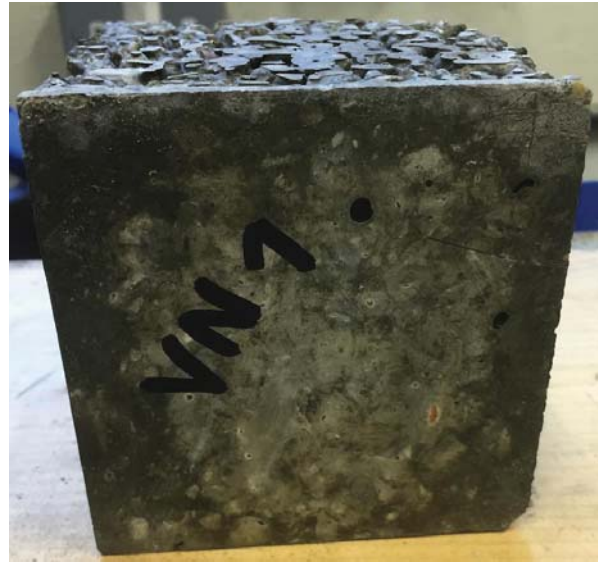
Fig. 5. Permeable concrete (a) as cast and (b) and rotated, showing the bottom is completely blocked by paste drain down, due to excessive cement paste content, w/c ratio and/or compaction. The sample is a 100 mm cube.
