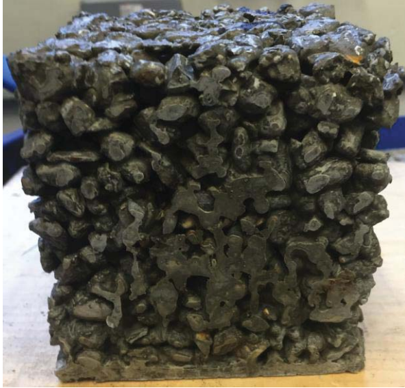
Fig. 5. Permeable concrete (a) as cast and (b) and rotated, showing the bottom is completely blocked by paste drain down, due to excessive cement paste content, w/c ratio and/or compaction. The sample is a 100 mm cube.
