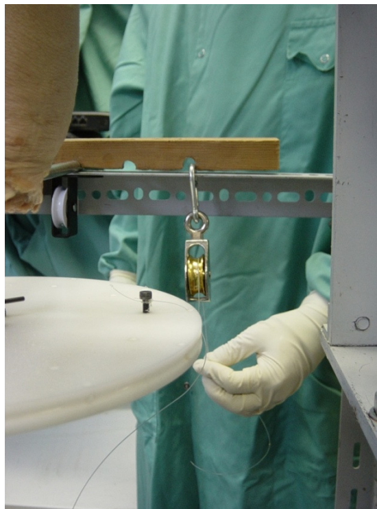
Figure 45: The grooved nylon rotation disc, box frame and pulley assembly. Note that the pull of the monofilaments was at the same level as the pulleys so that they ran parallel to the ground when applying rotational torque or varus / valgus load.
