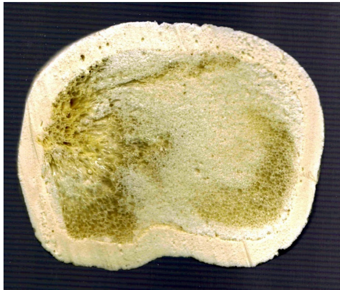
Figure 177: Scanned life size image of the tibial cut surface of an anatomical Sawbones (7) model of the human tibia following a 10 mm 0 degree resection as per the experimental and normal surgical protocols.
