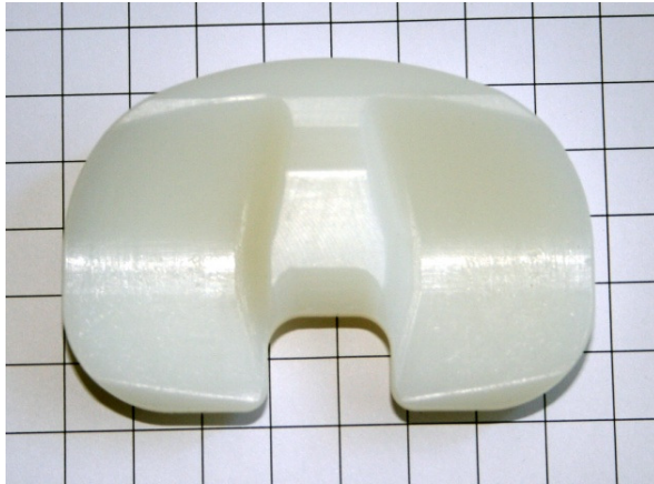
Figure 21: Photographs of a Stryker Scorpio CR polyethylene tibial insert.
