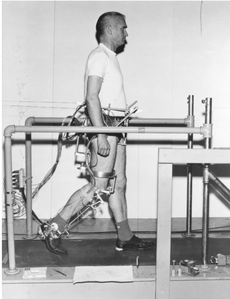
Figure 9: A photograph of the exoskeletal goniometer as used in the pioneering work and subsequent thesis “Experimental Kinematics of Human Walking”, University of California at Berkeley, 1970 (6) .
