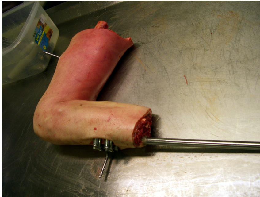
Figure 64: Photograph of calibrated and resected specimen with tibial rod cemented in, prior to femoral potting.
