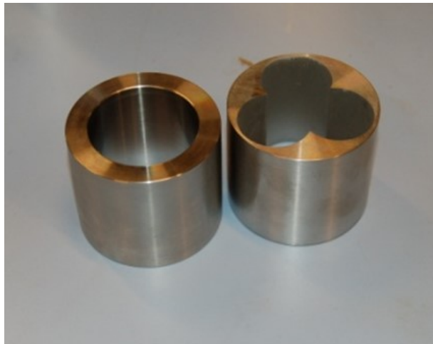
Figure 3.6: Volume reducing cylinders placed in the ageing cell's vessel.
