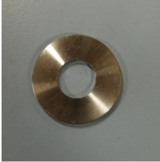
Figure 3.5: Metal insert to reduce the volume of the ageing cell's vessel.
