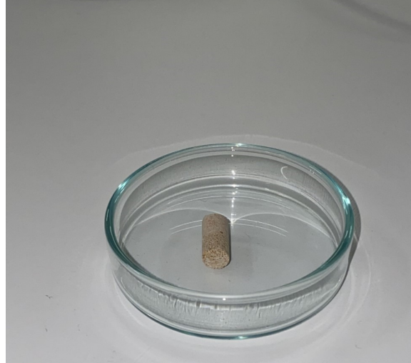
(b) Ketton rock sample drilled out of the main cylinder to a suitable size for AFM imaging.
