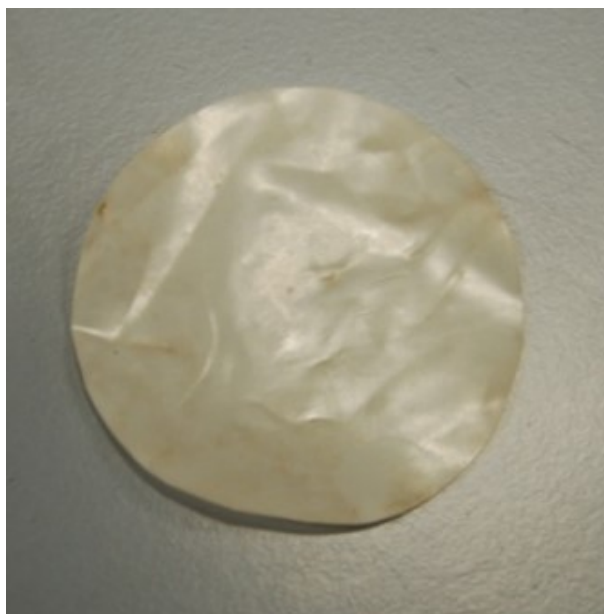
Figure 3.7: Teflon disc to avoid capillary contact between rock plugs.
