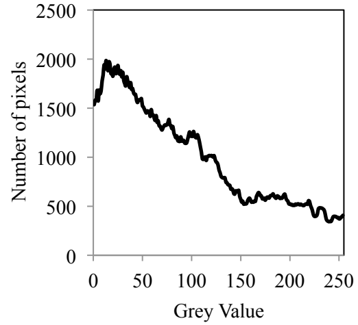
(b) Brightness histogram of pore distance map from spacer boundary (Figure 5.8e). The grey value 0 (black) representing the solid phase is not plotted.
