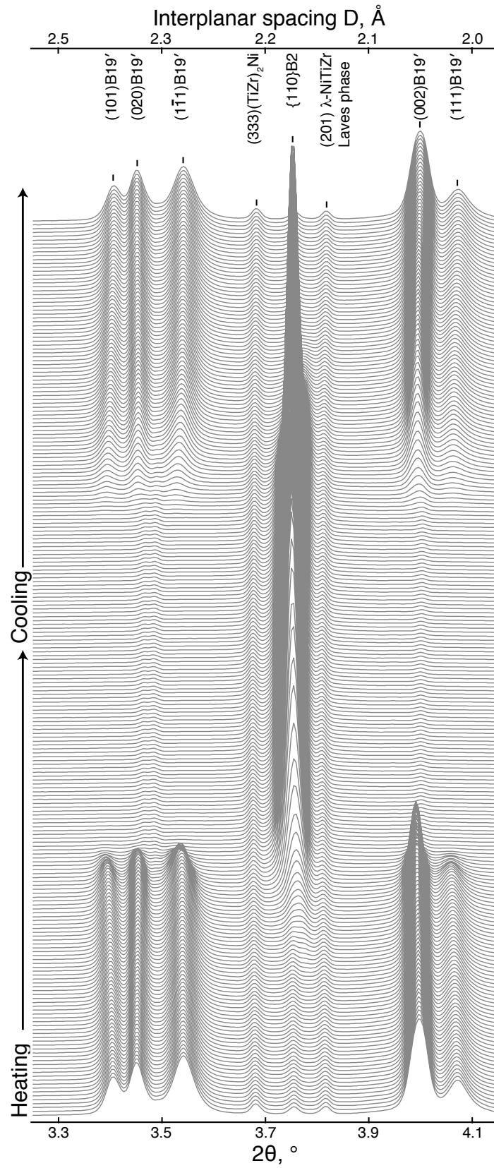
FIGURE 3.2: Evolution of the diffraction patterns during a complete heating and cooling cycle in Ni_{50}Ti_{35}Zr_{15} , showing the minor phases observed and the main B2 \leftrightarrow B19' transformation
