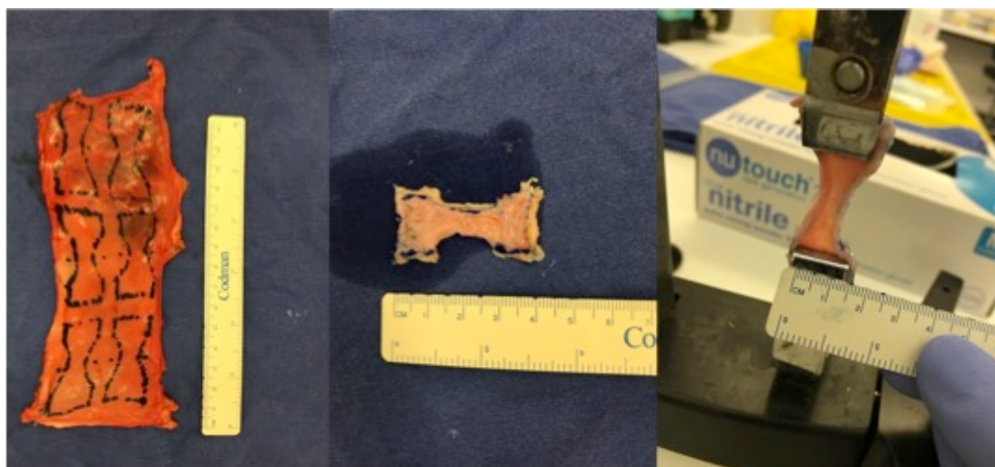
Figure 4.10: A demonstration of mechanical strength and strain testing using a tensiometer.
