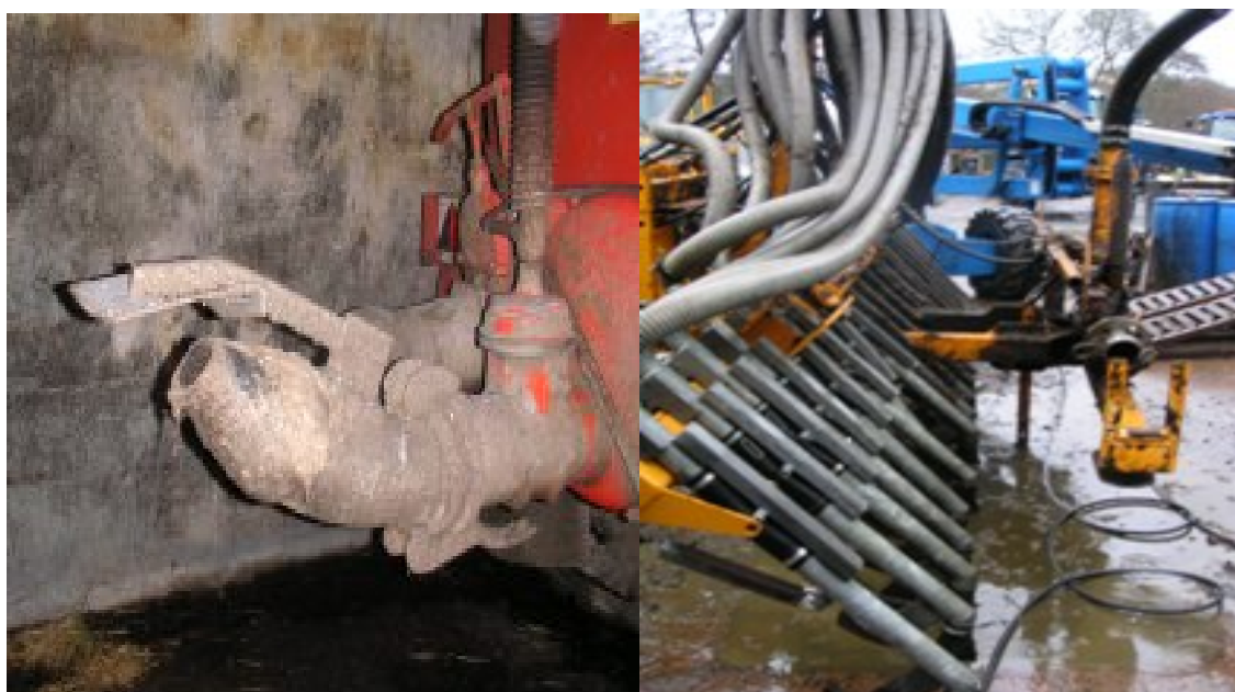
Plate 2.1 Slurry application equipment: (a) traditional 'splash-plate' (b) 'dribble-bar'.
