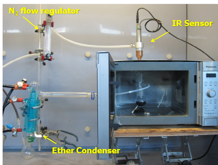
Figure 5.2. Modified domestic microwave system II
