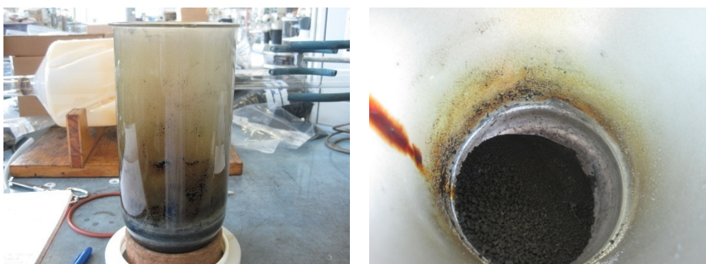
Figure 5.21. RotoSYNTH reactor after pyrolysis
