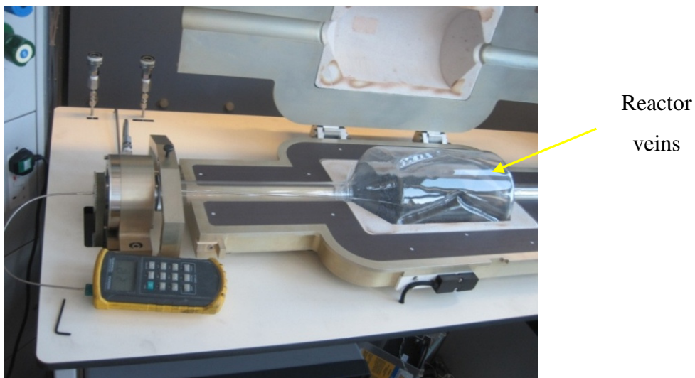
Figure 5.14. Thermocouple measurement of the SiC mix
