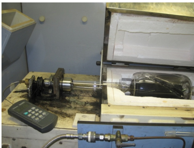
Figure 4.14. Thermocouple measurement configuration
