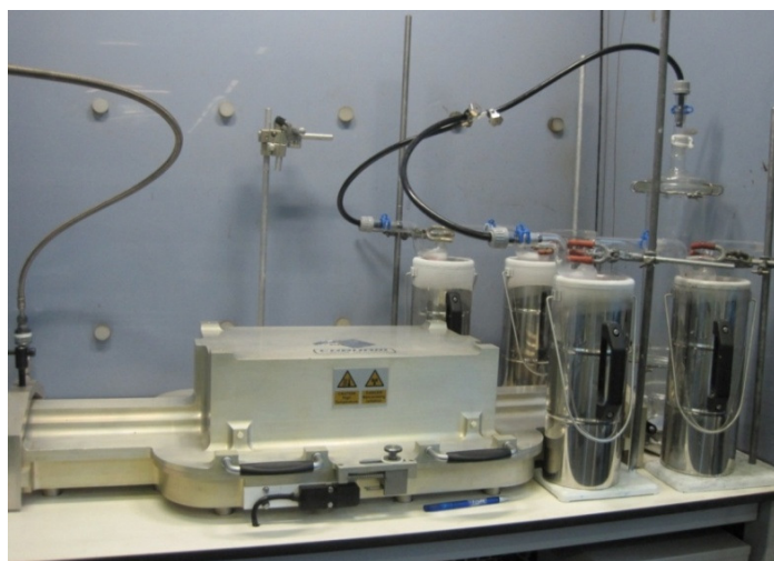
Figure 5.12. Condensation system using liquid nitrogen traps
