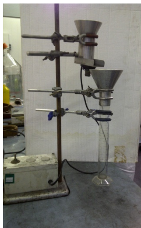
Figure 5.5. Apparatus for measuring apparent density
