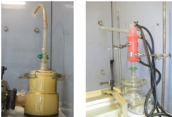
Figure 5.11. First two attempts for efficient condensation system
