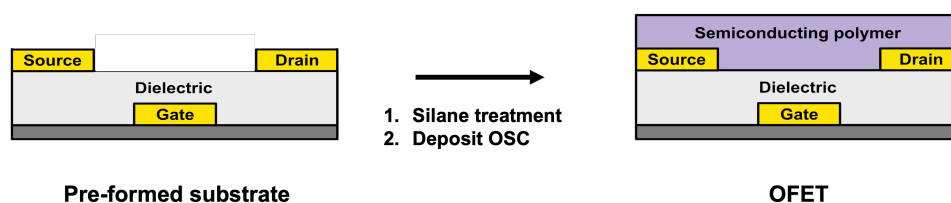
Figure 3.12: Illustration of OFET fabrication on the pre-formed Si/SiO 2 substrates.
