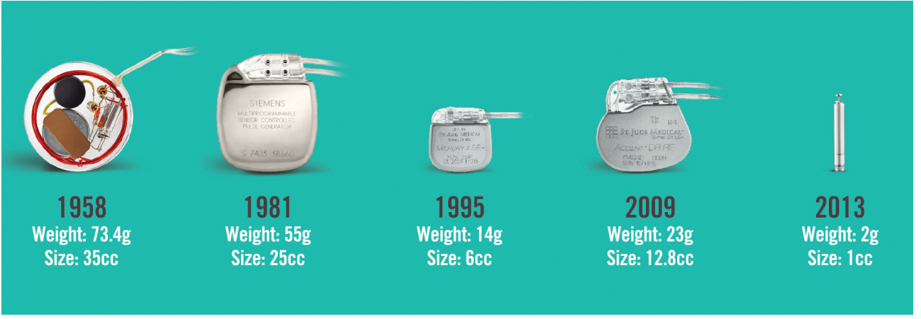
Figure 2.1: Evolution of implantable cardiac pacemakers since the first AIMD for heart conditions.
