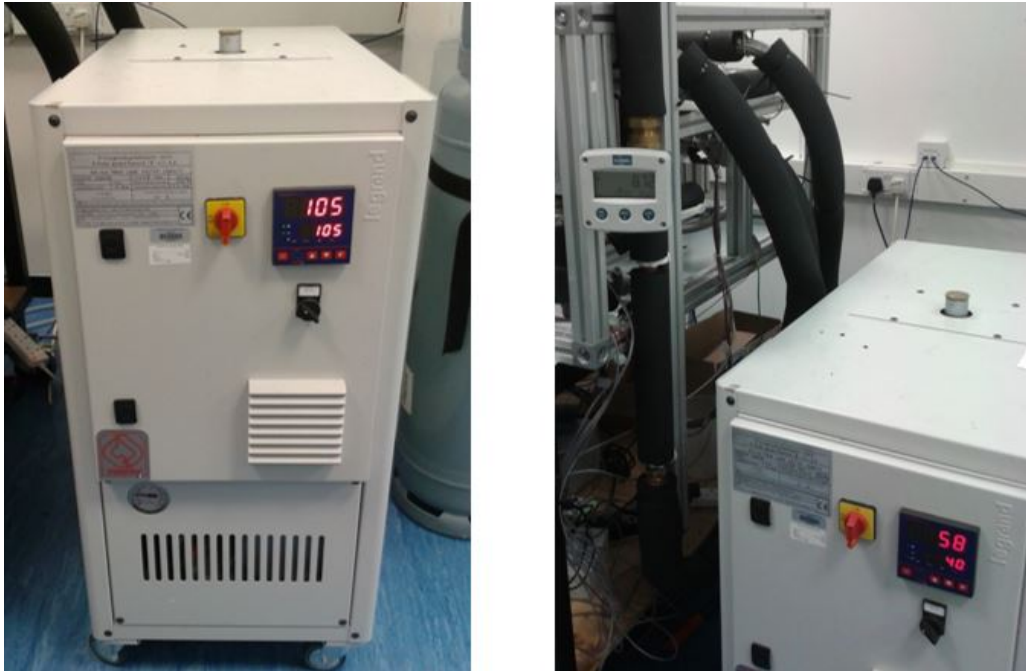
Figure 6.2: 18 kW electric oil heater used as heat source for the ORC test bench, delivering heat source temperatures in the range 100 – 120 °C. Also shown (right) is the turbine flow meter measuring thermal oil flow-rate through the evaporator.
