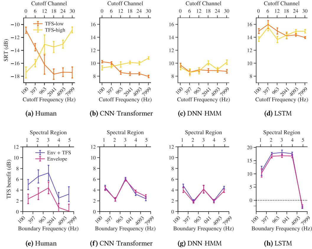
Figure 6.3. Performance in the two TFS experiments measured on 100 IEEE sentences (20 per SRT, 5 per condition) in six-speaker babble noise. In these experiments, TFS is either removed or retained in specific frequency channels using a tone vocoder. This vocoder initially filters speech in 30 frequency channels. To remove TFS from a given channel, the channel response is replaced by a tone that is modulated by the channel envelope. Human reference data, which was measured on the CRM task corpus (Bolia et al., 2000) in single-speaker babble noise, was taken from K. Hopkins and Moore (2010). Error bars are plotted at standard error of the mean. (a-d) In the first experiment, TFS information is added cumulatively starting either from the highest ( TFS-high ) or lowest ( TFS-low ) spectral region. The SRT-70.1s are plotted as a function of cut-off region for each of these conditions. Note that at both the highest cut-off frequency in TFS-high and lowest cut-off frequency in TFS-low , the whole sentence is vocoded. Conversely, TFS information across the whole frequency spectrum is present at the lowest TFS-high region and highest TFS-low region. (e-h) In the second experiment, TFS information was either removed or retained in a given spectral region, while all other regions were vocoded. A third condition was also measured in which the spectral region was completely removed. The benefit of adding envelope information was calculated as the difference between the SRT for the condition in which all regions were vocoded (i.e. TFS was removed in that region) and the SRT for the condition in which the spectral region was removed from a fully vocoded sentence. The benefit from adding envelope and TFS information together was calculated as the difference between SRT for the condition in which the spectral region was removed fully and the condition in which TFS was retained.
