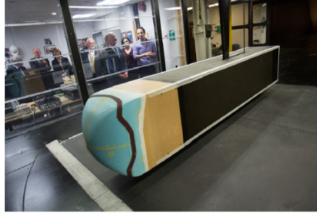
Figure 5.1: Simplified lorry model used for wind tunnel experiments (Cabitza (2013)).
