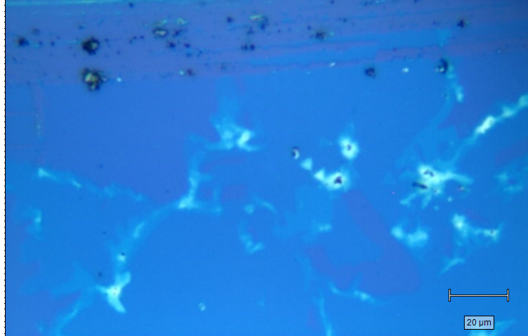
Figure 10.3: Optical micrograph of WS_2/MoS_2 heterobilayer on SiO_2/Si
