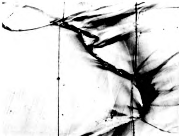
FIG. 4.14a. Apparent offsets in scribed markers. T = 21^{\circ}\text{C} Specimen M4 at 0.9% strain. (X 290).
