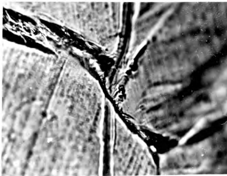
FIG. 4.14b. Part of same area as in fig. 4.14a showing curvature of marker at boundary. (X 1390).
