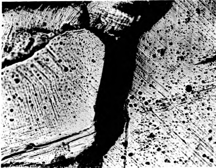
FIG. 4.9. Cracking at grain boundary. Specimen MX8 at 8.76 % strain. (X 200).
