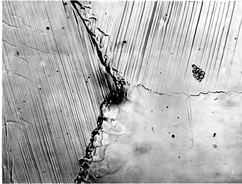
FIG. 4.25. Internal polygonisation. Specimen MX 21 at 8.89% strain. (X 325).
