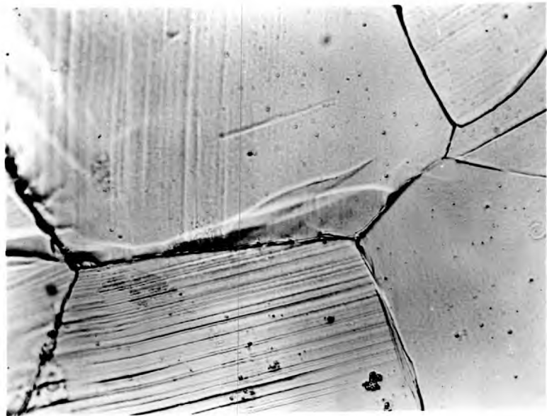
FIG. 4.23. Grain boundary configuration at surface. Specimen MX 31 at 5.18% strain. (570).
