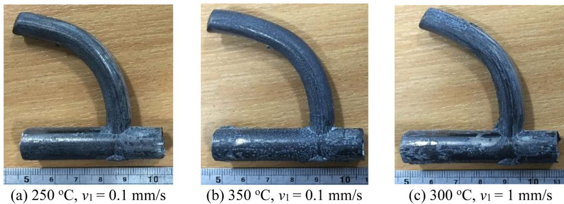
Fig. 4. AZ31 profiles extruded at velocity ratio v_2/v_1 = 1/2 and different temperatures and strain rates.
