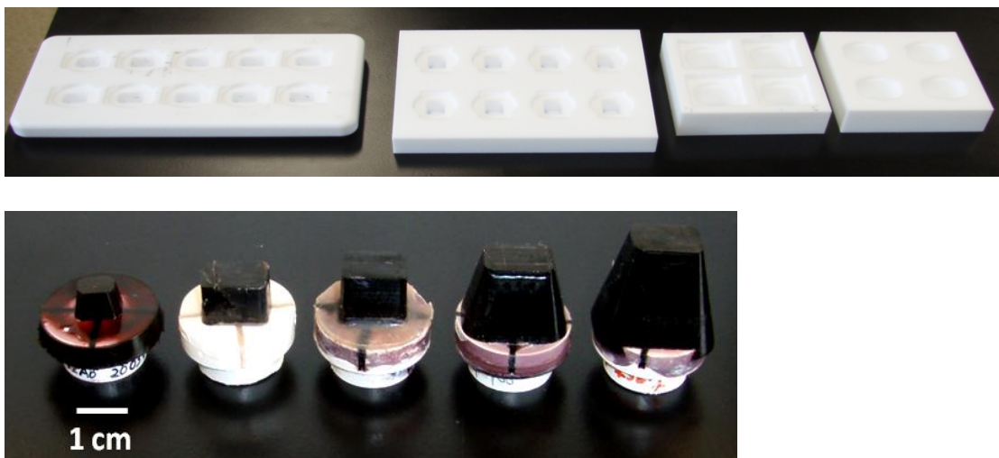
Figure 2-4: Embedding moulds and embedded samples. From the left hand side, depth of the mould is 8, 12, 15 and 20 mm, respectively. Embedded samples are dark wine red.
