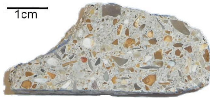
Figure 3.9: Flat section of small block sample SB1. Dimensions are 4.4cm by 2.3cm
