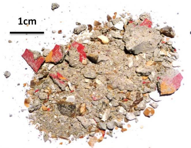
Figure 3.8: CONSORT bioshield concrete sample. The red pigments are from the outer paint layer of the shield.
