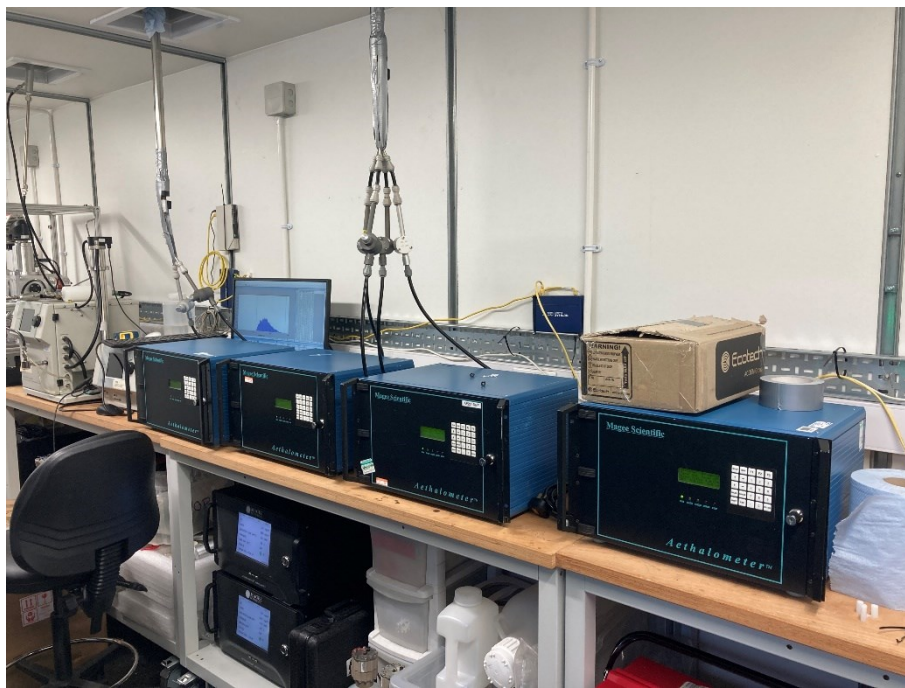
Figure 24 Aethalometer AE22 (top shelf) and AE33 (bottom shelf) installed at Honor Oak Park site cabin during second comparison campaign in 2022 (source: personal collection).
