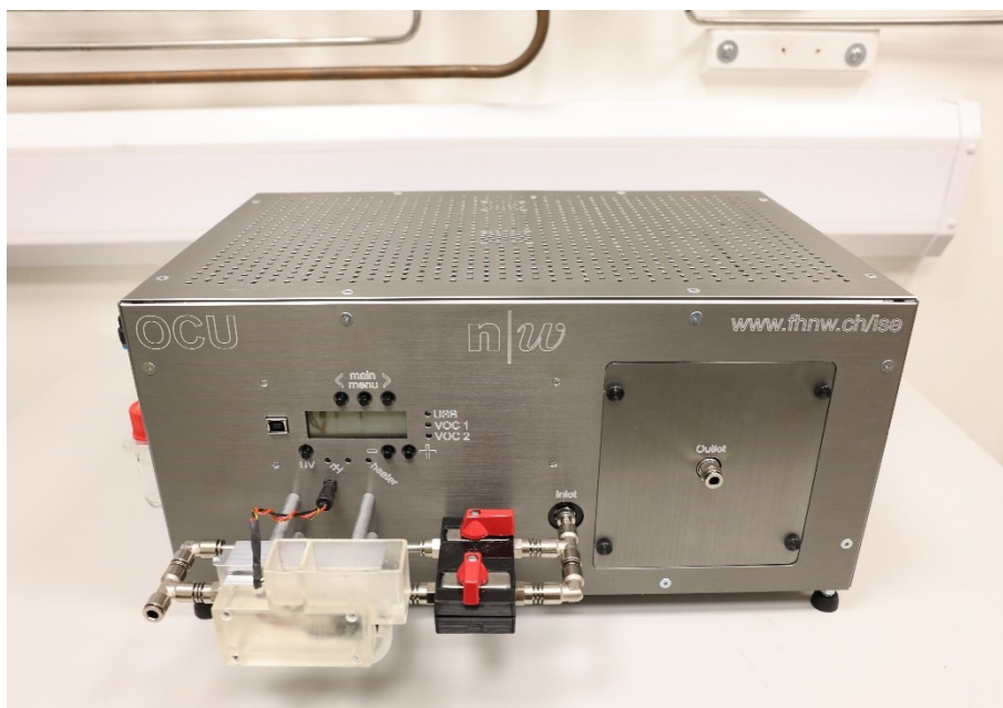
Figure 2 Organic Coating Unit (OCU) used in this study (source: NPL).
