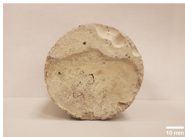
Figure 5.11 Bottom surface of a typical M spacer showing an uneven base
