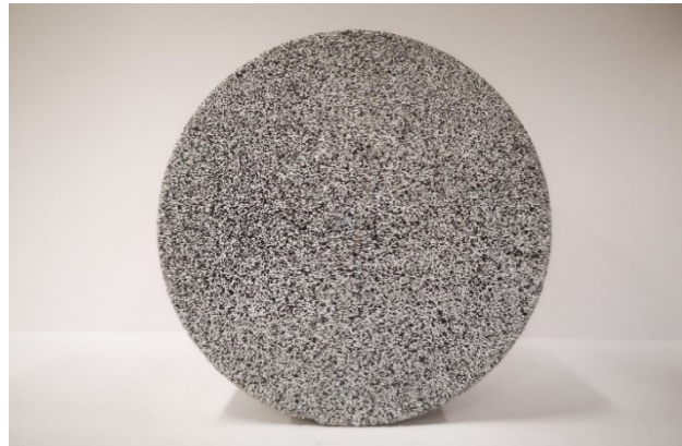
Figure 3.6 Speckled sample for DIC
