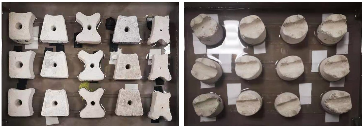
Figure 4.5 Water sorptivity test setup
