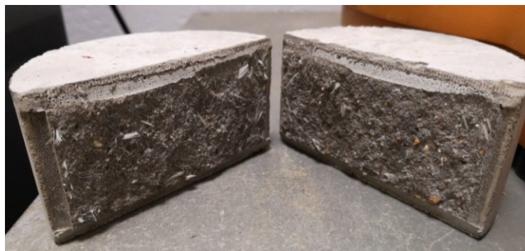
Figure 3.2 Fibre-reinforced mortar split using the optimal groove orientation and loading regime
