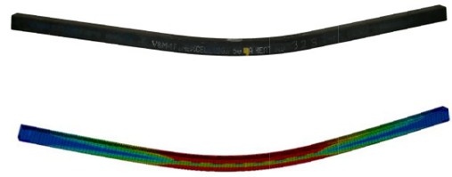
(b) S690 SHS 50×50×5 under four-point bending
