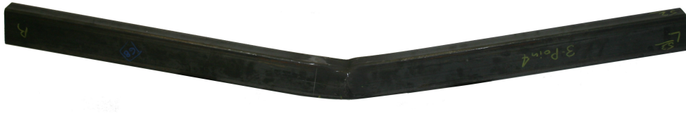
Figure 8: Typical three-point bending failure mode (S460 RHS 100 × 50 × 4.5).
