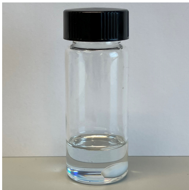
(b) 1:2 CAGE, dried at room temperature, after being stored at −20 °C for 6 months.
