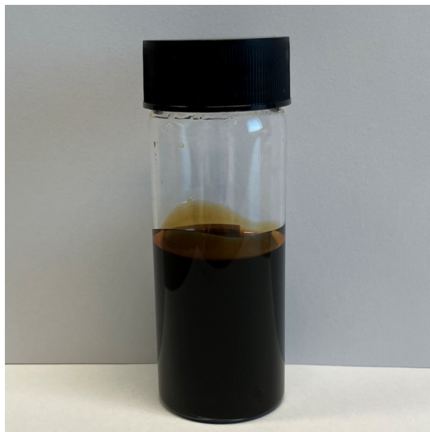
(b) 1:2 CAGE dried at 40 °C for 24 h, then stored at room temperature for 6 months.
