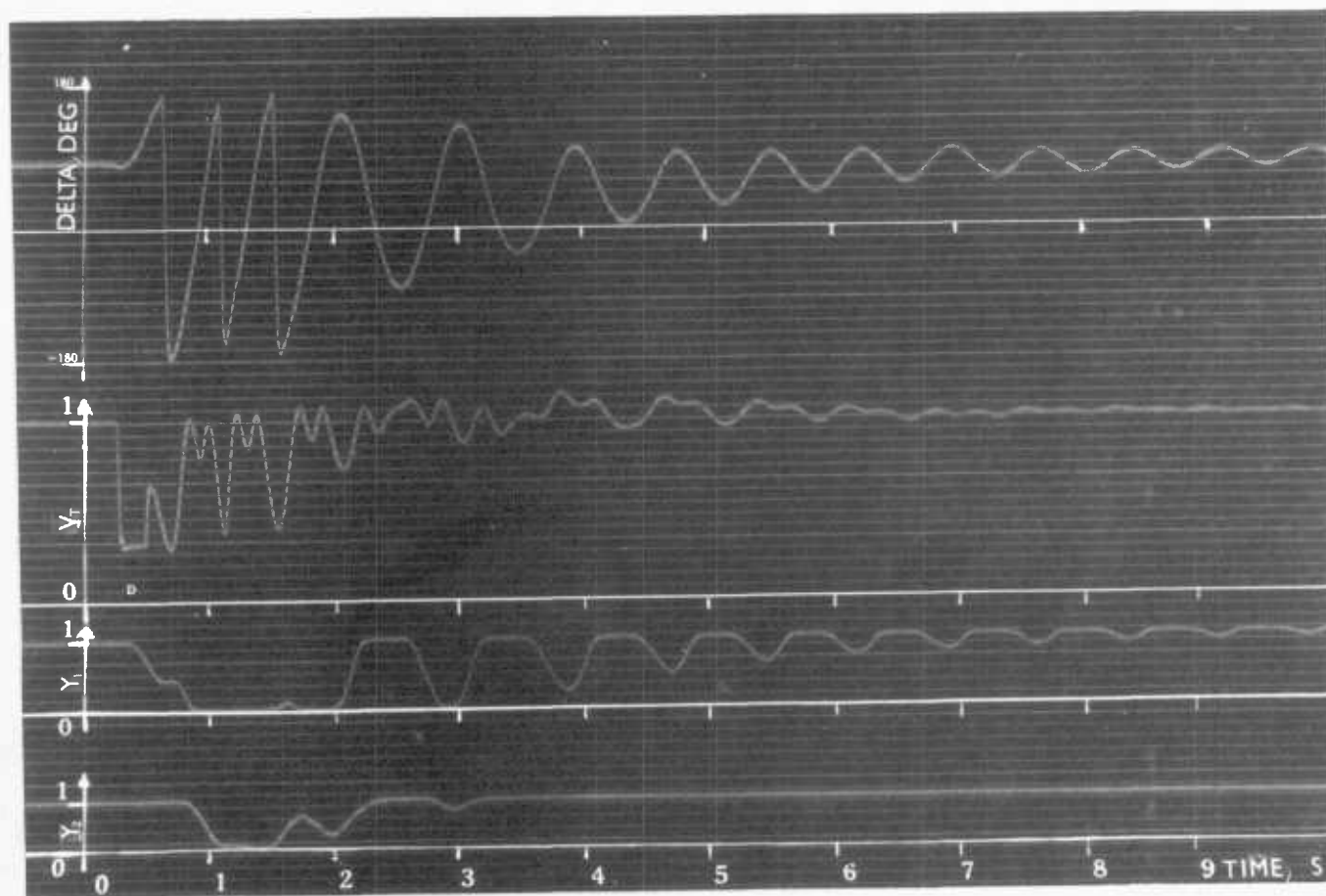
FIG. 5.8 MICROMACHINE SIMULATION OF NORTHFLEET TEST No. 6 V_T MICROMACHINE TERMINAL VOLTAGE Y_1 THROTTLE VALVE POSITION Y_2 INTERCEPTOR VALVE POSITION RELAY OPENING TIME CONSTANTS = RELAY CLOSING TIME CONSTANTS
