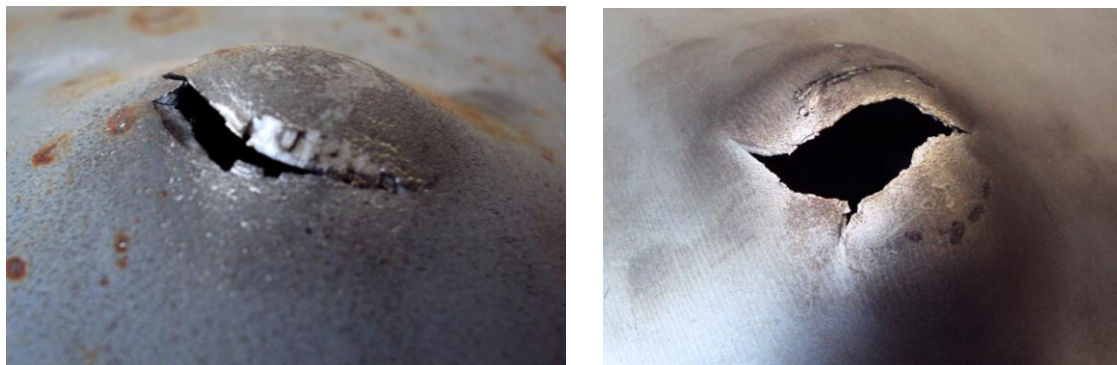
Figure 3-29: Panel rupture (left: armour steel; right: mild steel)
