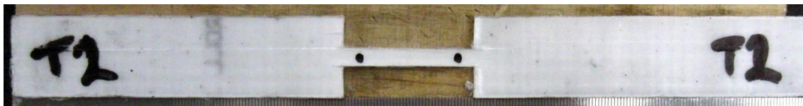
Figure 5-11: Reduced-width tensile specimen of Dyneema HB26
