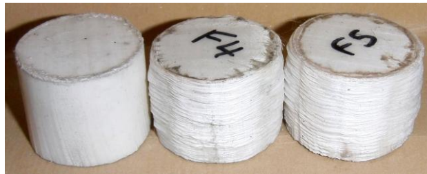
Figure 5-18: Pristine (left) and tested (middle, right) Dyneema HB26 samples after through-thickness compression tests
