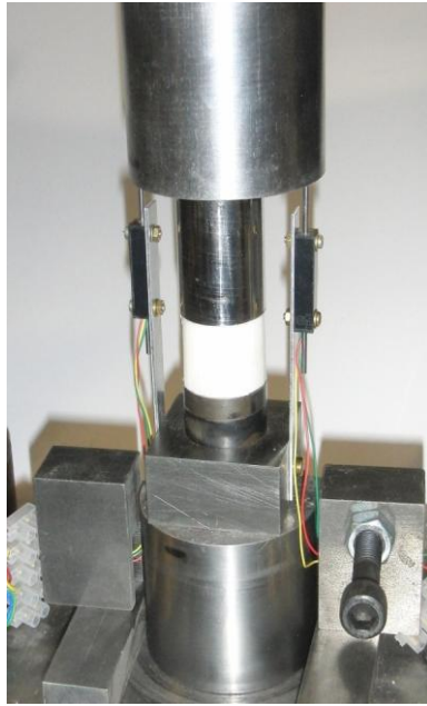
Figure 5-17: Through-thickness compression testing of thick Dyneema HB26 sample
