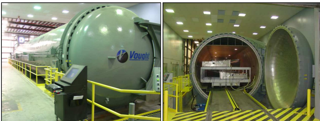
Figure 1.2. Autoclaves for creep age forming [27].
