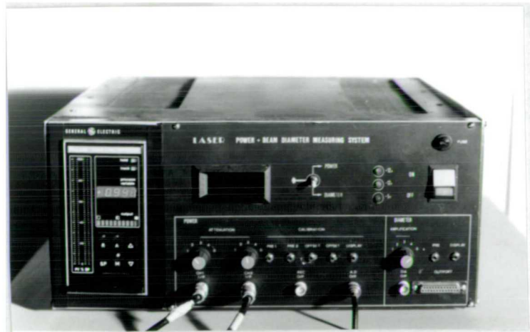
Fig. 5.30. Closed loop laser power controller instrument.
