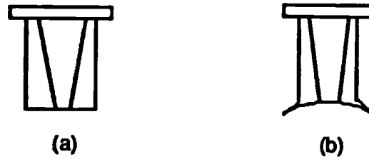
Fig. 4.13. Discription of the spherical nozzle for beam recycling and pre/post heating. a). ordinary nozzle. b) spherical nozzle.
