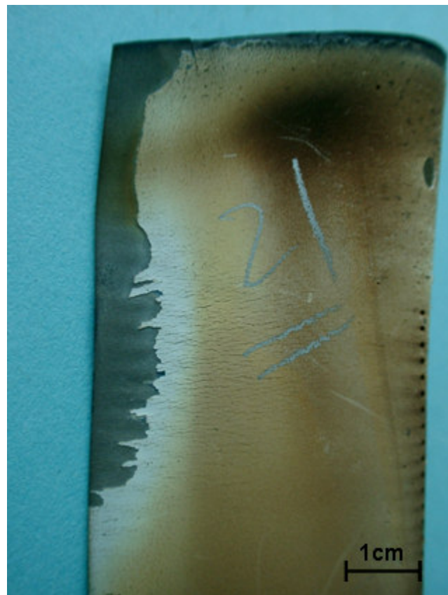
Figure 58 Blade #1 white surface observed right next to TBC failure site
