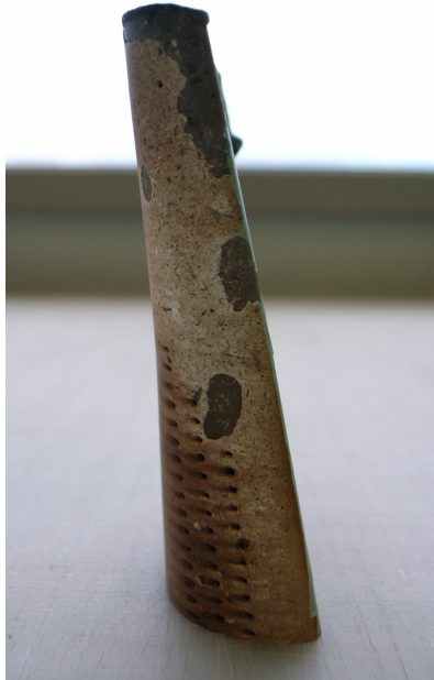
Figure 61 Spallation of TBCs on the suction side leading edge of blade #1
