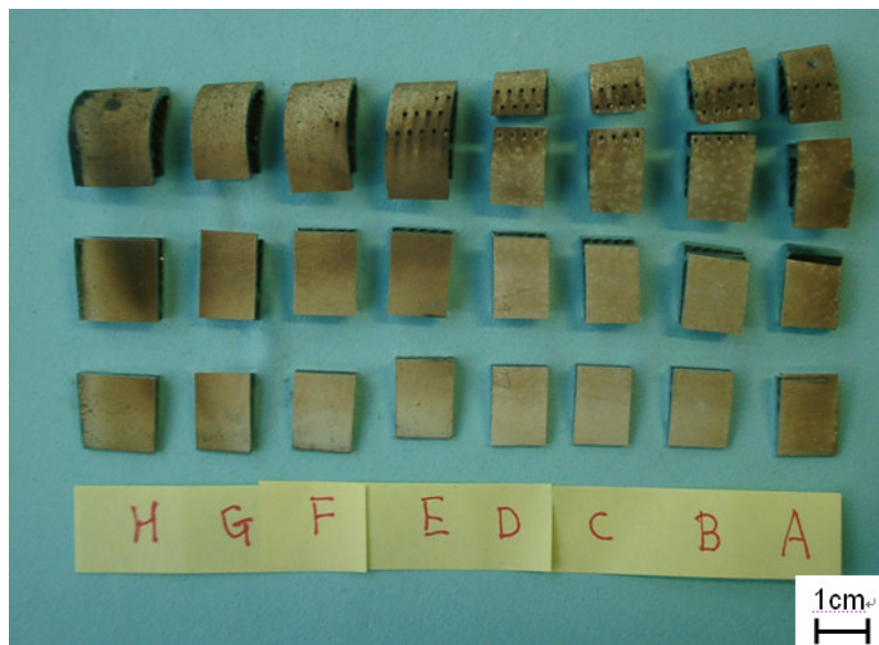
Figure 55 Blade #2 is divided into 8 horizontal sections and 28 pieces
