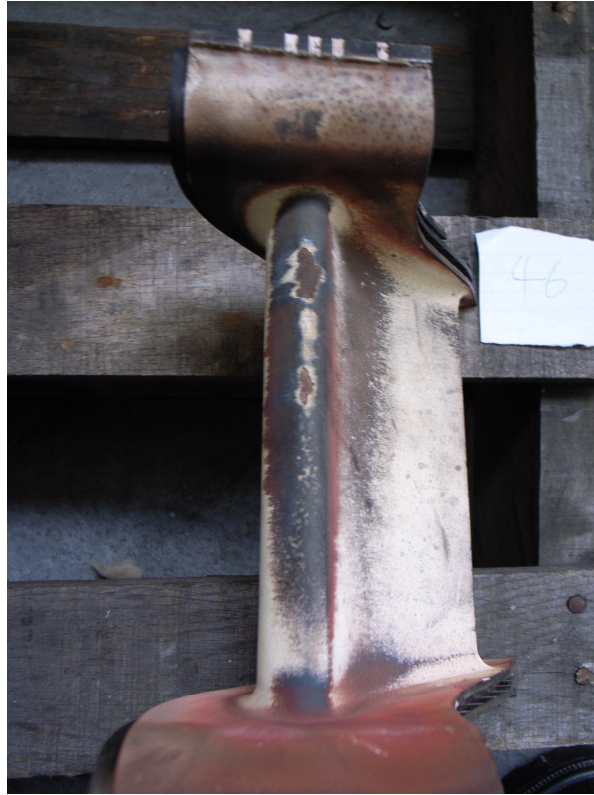
Figure 25 Spallation of Vane C on the pressure side leading edge
