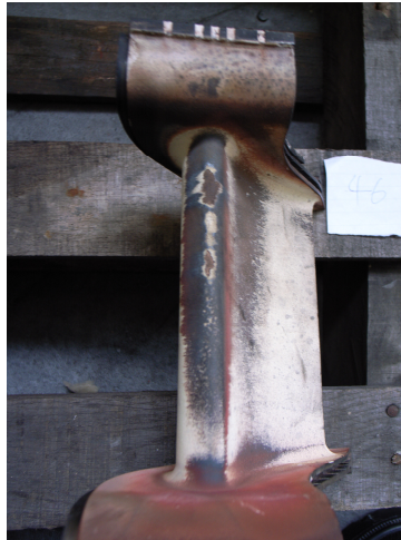
Figure 3 Spallation of Vane C on the pressure side leading edge
