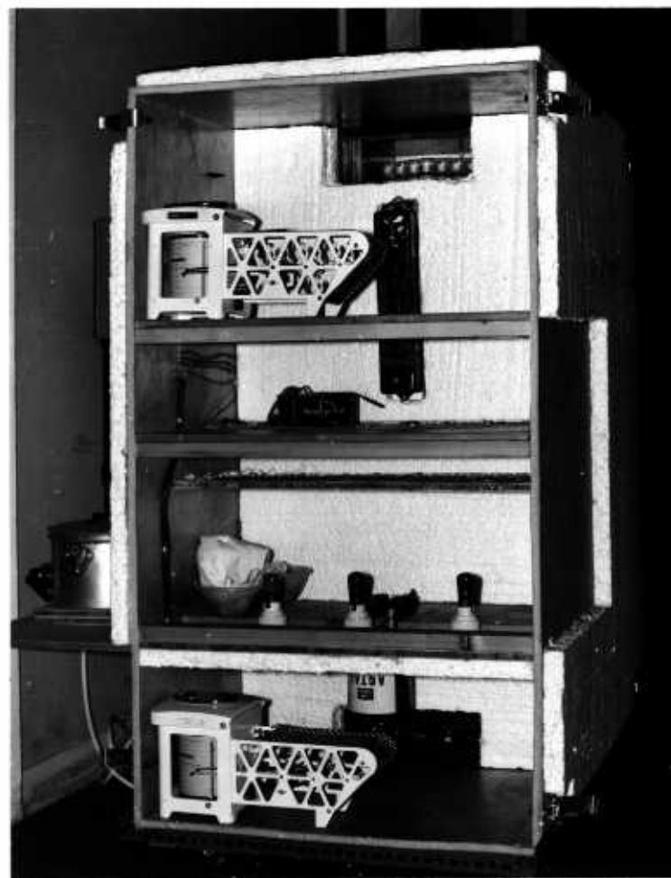
Figs. 8c and 8d The air-conditioning end of the irradiation cabinet showing the door closed and open. The apparatus controlling the temperature and humidity is described in chapter 8.2.2.
