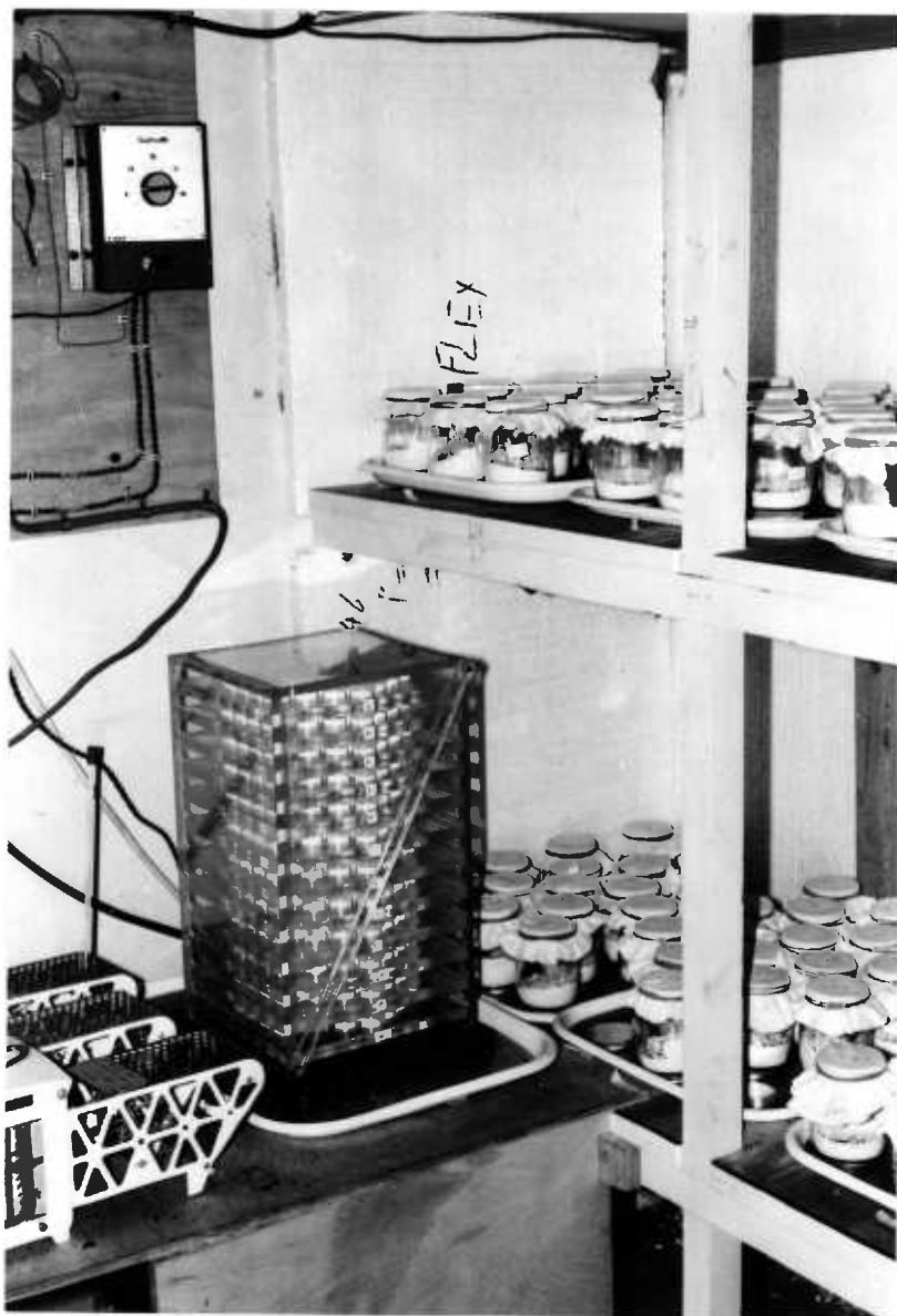
Fig. 8b One corner of the constant-temperature room. The glass honey-jars containing irradiated weevils and flour can be seen standing on small platforms in the oil filled trays on the right hand shelves. The perspex nest of shelves in the centre of the picture was used to house specimens during irradiation in the specially designed irradiation cabinet described later (8.2).
