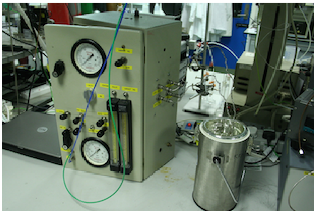
Figure 3.11: Downstream FRT System
