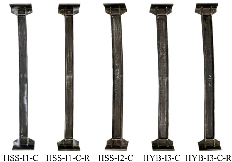
Figure 3.13: Failure modes of tested welded I-section columns
