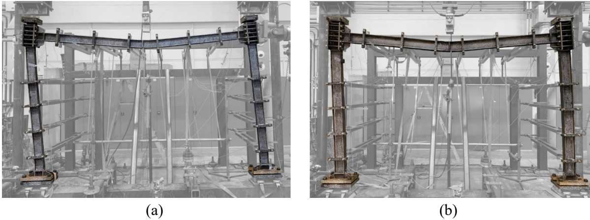
Figure 6.21: Failure modes of tested frame specimens subjected to the second combination of horizontal and vertical loads (a) HSS-I-65×116-V&H-2; and (b) HSS-I-80×136-V&H-2.
