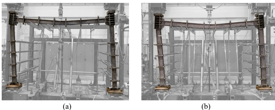
Figure 6.20: Failure modes of tested frame specimens subjected to the first combination of horizontal and vertical loads (a) HSS-I-65×116-V&H-1; and (b) HSS-I-80×136-V&H-1.
