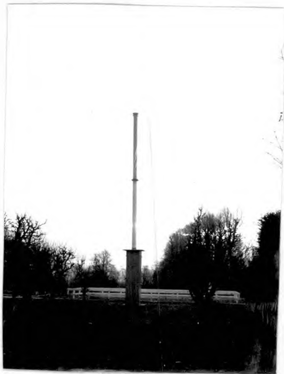
FIG. 2.3. The suction trap
